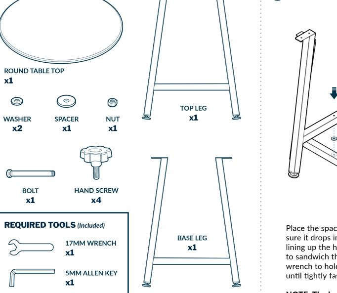
Place the spacer on top of the base leg crossbar, and make sure it drops into place. Then, place the top leg on the spacer, lining up the holes. Line up the bolt, washers, and nut in order to sandwich the legs and hold everything in place. Using the wrench to hold the nut still, turn the bolt with the Allen Key until tightly fastened.
