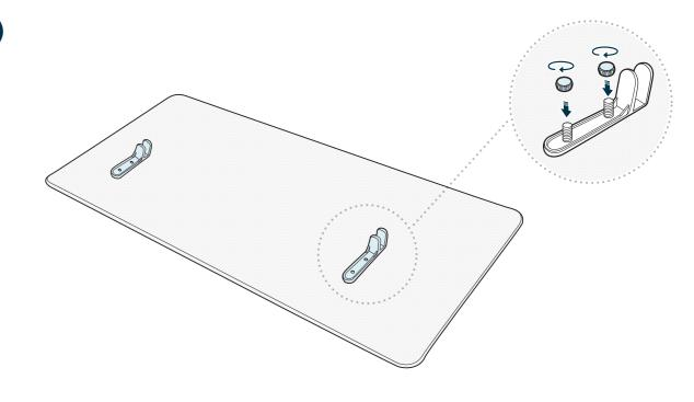
Screw on the bolt caps and tighten until the bracket is firmly affixed to the panel.
