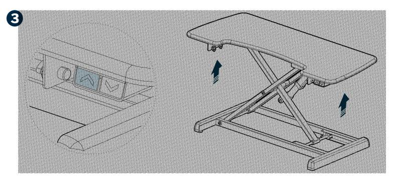
With the converter plugged in, press the up arrow button until the converter is raised to its highest position, providing room to attach the keyboard tray.
