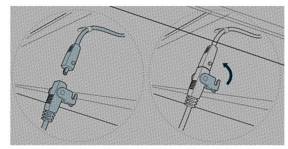
Locate the pre-installed power cord underneath the back of the converter's top tray. Join the power adapter cable to the pre-installed power cord, then secure the connection by latching the hook. Plug the converter into an outlet.
