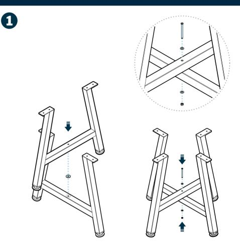
Place the spacer on top of the base leg crossbar, and make sure it drops into place. Then, place the top leg on the spacer, lining up the holes. Line up the bolt, washers, and nut in order to sandwich the legs and hold everything in place. Using the wrench to hold the nut still, turn the bolt with the Allen Key until tightly fastened.
