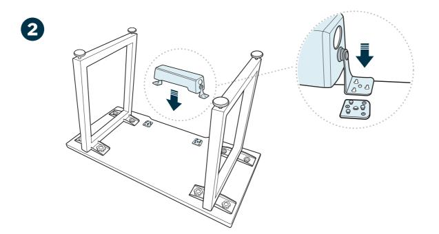
Slide the cable management tray into the notches at the edge of the table and push until it clicks, indicating it is locked into place.
