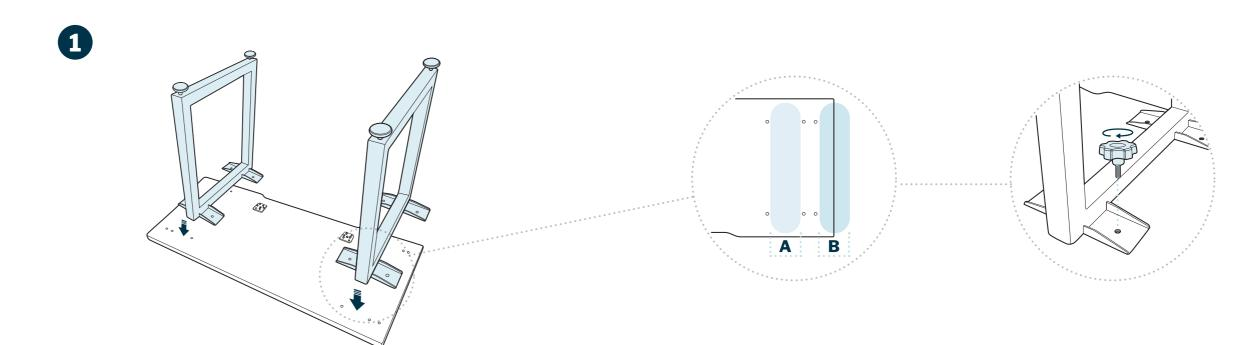
Table top and table legs will arrive in separate boxes. We recommend assembling the table face down in the box to prevent any surface scratching. Unbox the legs and line up legs with desired connection points.
