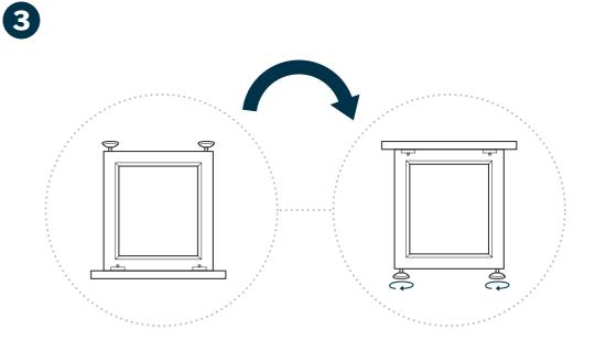
Two people should lift and flip the assembled table to an upright position. Adjust the footpads to level table as needed.
