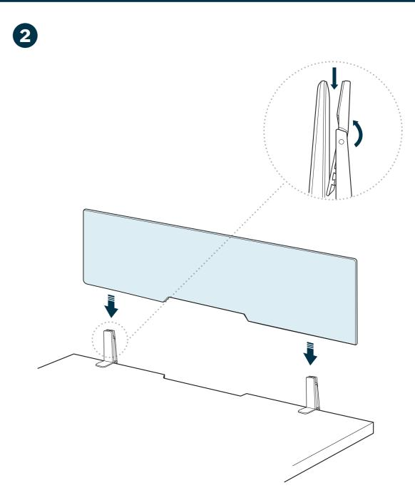
Carefully slide the acrylic panel all the way down into the brackets.
