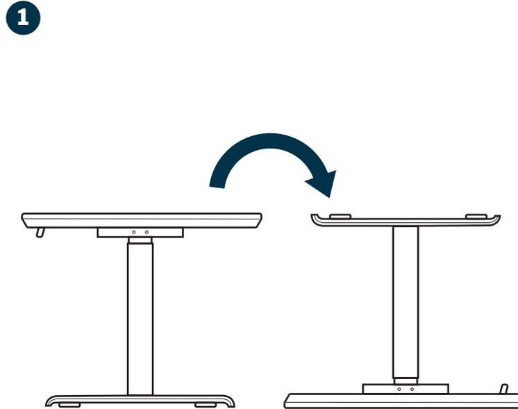
If this is an accessory add-on and the desk is already assembled in the upright position, you'll need to flip the desk over to properly attach the cable tray. First, ensure the work surface is free from hard debris that could damage the table surface, then lower the desk edge opposite the control panel onto the floor before flipping the desktop face down.
