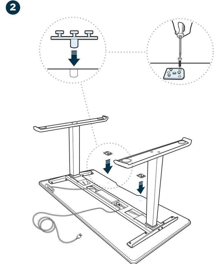
Align the cable tray brackets over the pre-drilled holes and dowel hole (at the edge of the desktop opposite the control panel) and use screws to attach each bracket.
