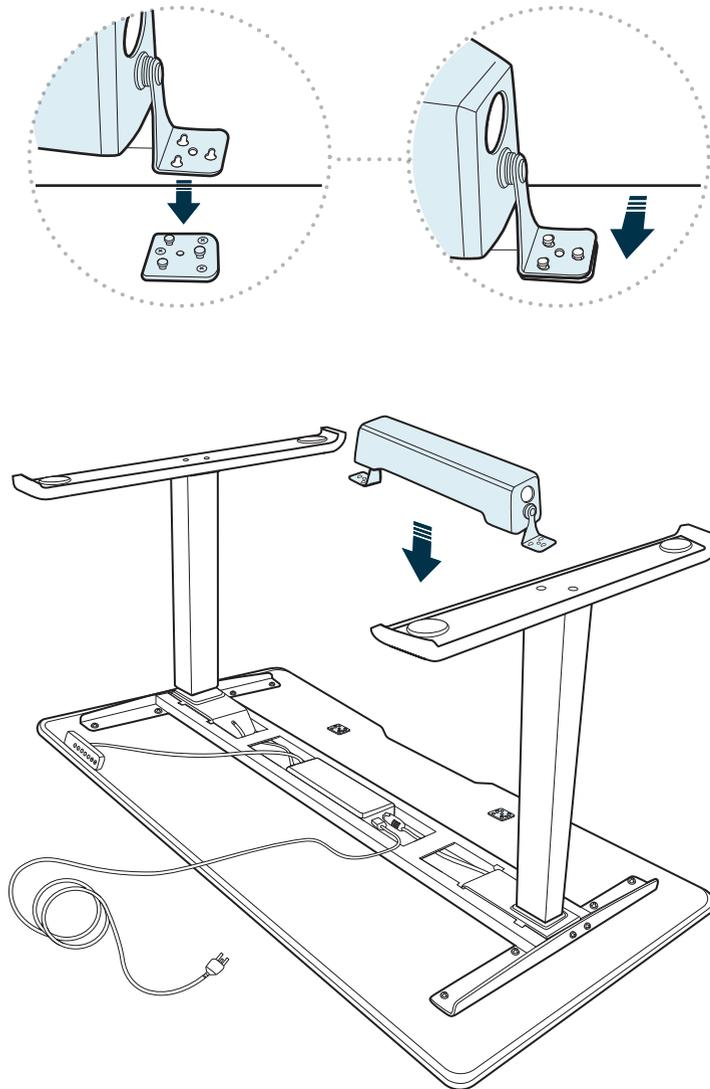
Lower the notches on each end of the cable tray over the brackets, and slide the tray (either toward the front or back of the desk) until they click into place. Run the power cord through the cable tray.
