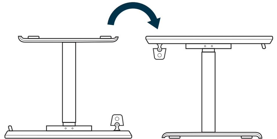
Once the cable tray is properly secured, flip the desk (along the edge opposite the control panel) into the upright position. Your desk is now ready to use.
