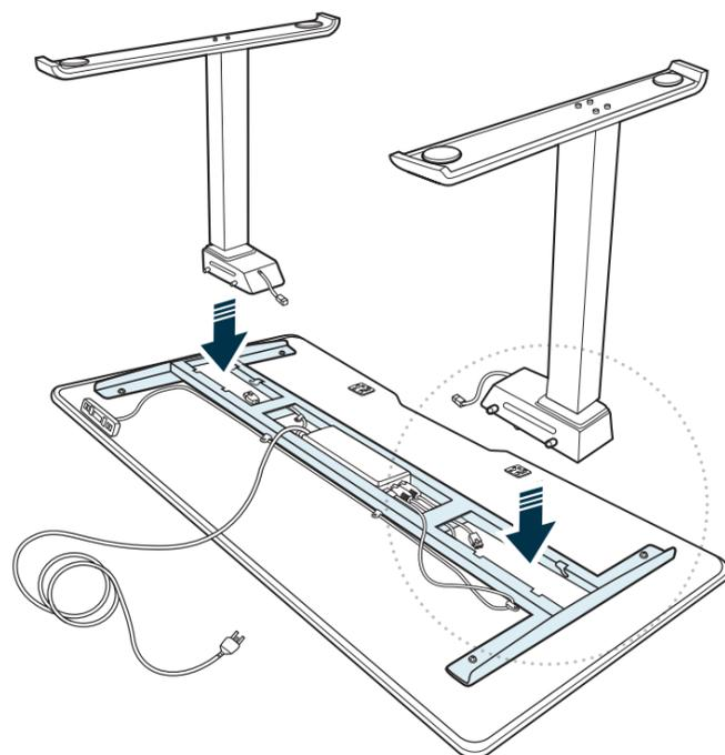
Desktop and desk legs will arrive in separate boxes. We recommend assembling the desk with the desktop face down in the box to prevent any surface scratching. Open the desktop box. Remove the desk legs from their box. Each leg is marked with (L) or (R). Place each leg into the grooved area on the corresponding side of the metal frame, with the longer section of the foot facing towards the front of the desk (the side with the straight edge and control panel).
