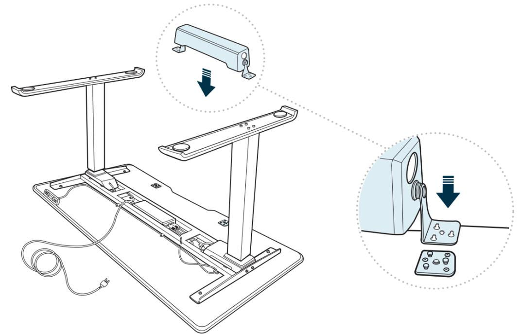
Slide the cable management tray into the notches above the bracket and push until it clicks into place. Run the power cord through the cable tray.
