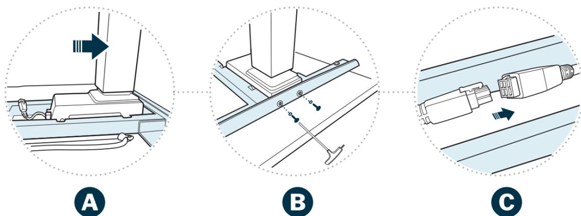
After each leg is placed into the grooved area, (A) push the leg all the way towards the outside of the frame. You will feel it click, confirming it's properly aligned. (B) Use the Allen key provided to securely tighten screws and washers onto each leg. (C) Connect the leg cable to the cable attached to the desk as shown and repeat for the other leg.
