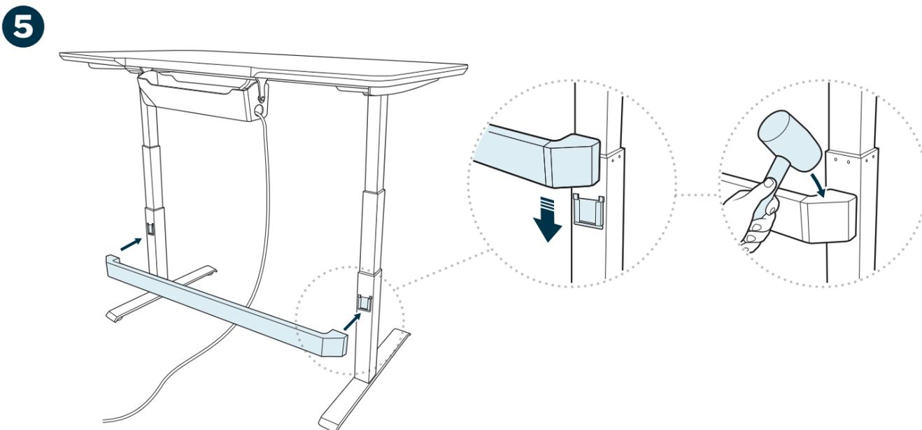
Once desk is fully raised, place the crossbar on the brackets on the back of each leg. Use the included mallet to hammer the crossbar down onto the brackets until the crossbar covers the brackets completely. You will know it is fully in place when the top of the crossbar reaches the red line.
