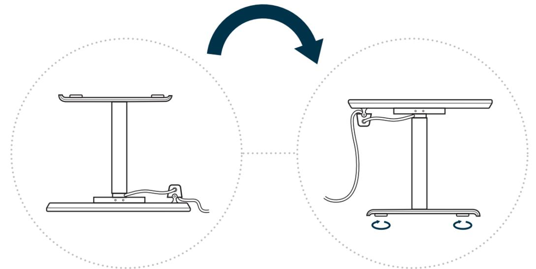
Once legs, tray, and power cords are secure, two people should carefully flip the assembled desk to an upright position. Adjust the footpads to level the desk as needed.
