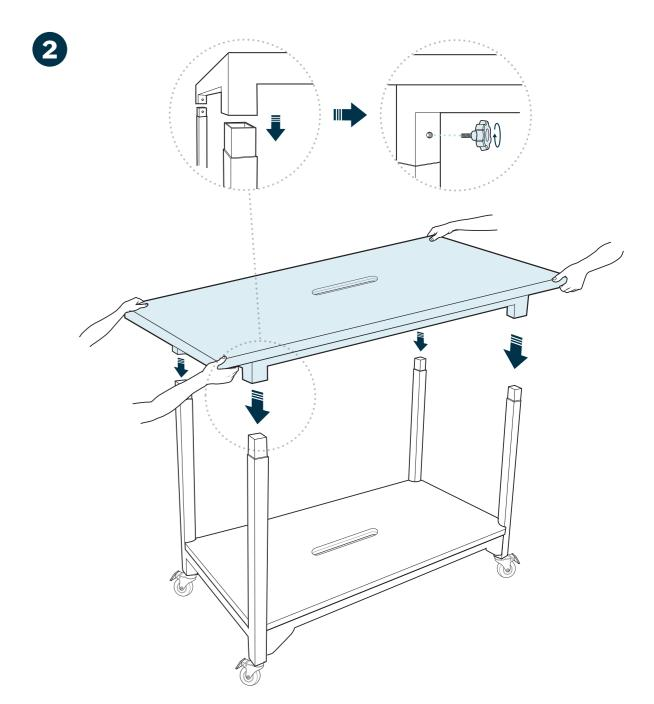
Have 2-3 people lift the top surface and line it up with the matching connection points on the tops of the legs. To avoid pinching fingers, hold the top surface by the corners. Once the connections are firmly placed, use the hand bolts to fasten the legs to the table top, and tighten until firmly in place.
